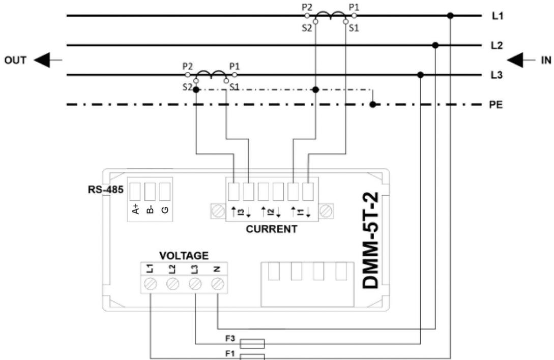
Fig. 5. 3P3W system – 3-phase, 3-wire system, semi-indirect-measurement
