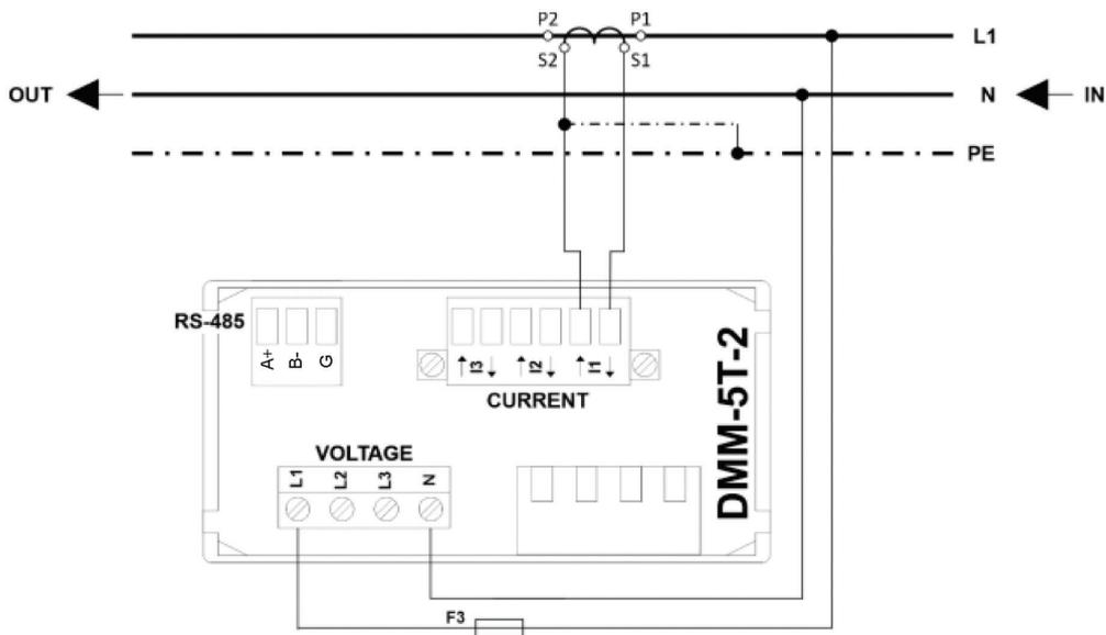
Fig. 3. 1P2W circuit – 1-phase, 2-wire system, semi-indirect-measurement
