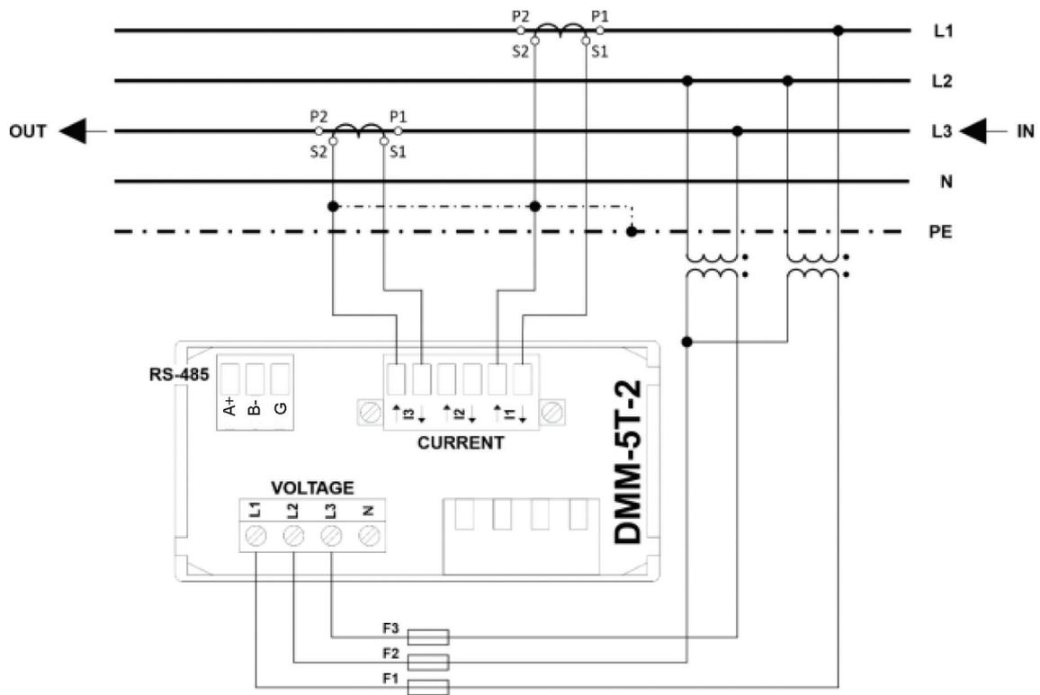
Fig. 7. 3P3W system –3-phase, 3-wire system, indirect measurement
