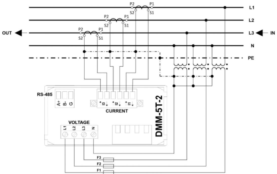
Fig. 6. 3P4W system –3-phase, 4-wire system, indirect measurement
