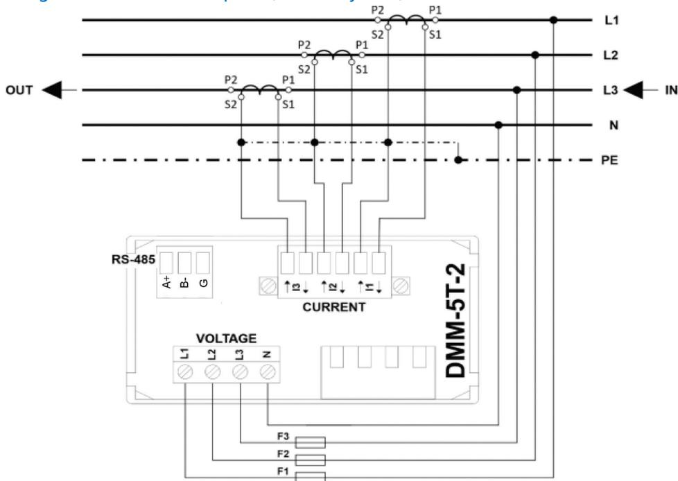
Fig. 4. 3P4W system – 3-phase, 4-wire system, semi-indirect-measurement
