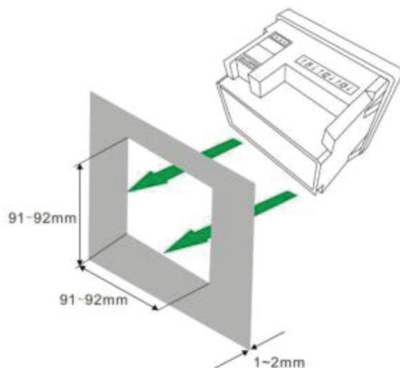
Fig. 1. Multimeter assembly method
